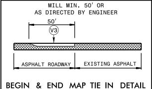
TIE ASPHALT OVERLAY TO EXISTING ASPHALT
